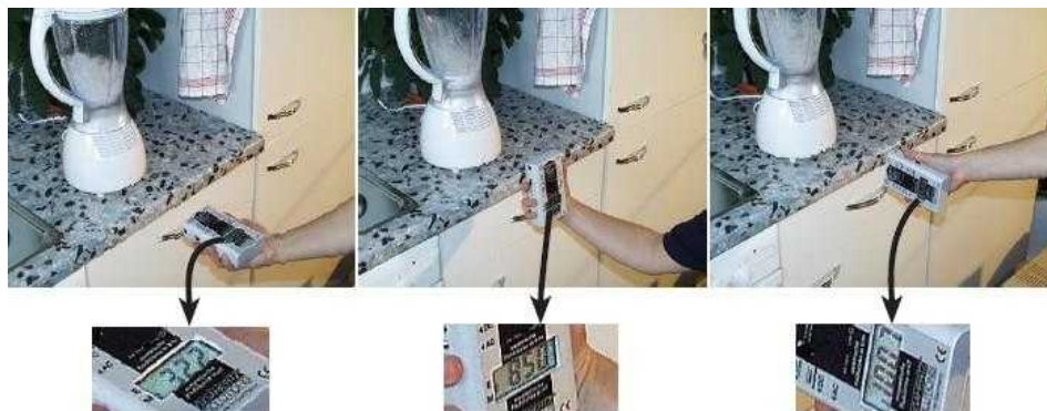
[그림 4-6] Three dimension measurement of field source
